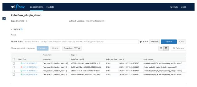
The UI presents the pipeline status (in form of the icon) and latest node that was run (for failed runs in indicates at what step did the pipeline fail). Also, the vertexai\_run\_id and vertexai\_job\_name tags can be used to correlate Mlflow run with the Vertex AI pipeline execution.
